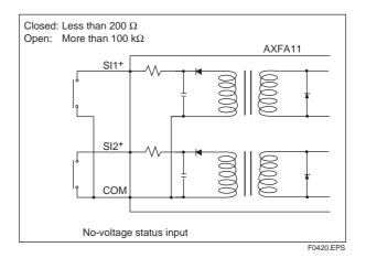
Figure 4.4.12 Status Input Connection
